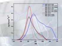
Comparative Peak Fit decomposition of the thermal signals: BSA (concentration = 7mg/ml) in the absence (black solid line) and in the presence of TiO<sub>2</sub> NP concentration = 0.00994 mg/ml (red line) or ZnO NP concentration = 0.0115 mg/ml (blue line) at three pH 7.4 buffer phosphate. Dash lines represent the corresponding PeakFit components.
